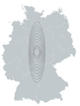
In the second case an ellipse is used specifically for HVDC projects with prioritised underground cabling, whose form tapers (HVDC ellipse) as the distance between two grid connection points increases. Conversely, the ellipse broadens, the closer two connection points are to each other.
