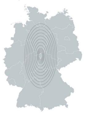
The geometric construction of the ellipses distinguishes between two cases (see Figure 1). In the first case an ellipse is used – as previously – whose minor axis (horizontal axis) measures half of the main axis (perpendicular axis) (2:1 ellipse). This is used for alternating current projects and for direct current projects for which priority is not given by law to underground cabling (currently BBPIG Project 2, Ultranet).
